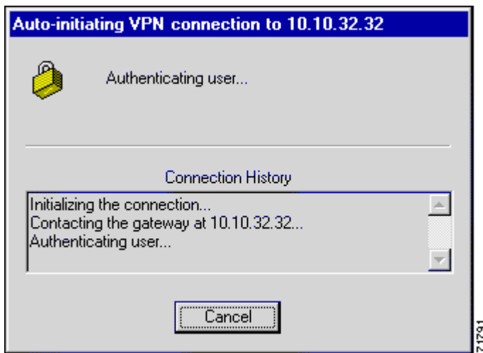
Figure 4-22: Viewing Dial Status of an Auto Initiated VPN Connection
